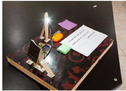
Phone charger by solar energy
